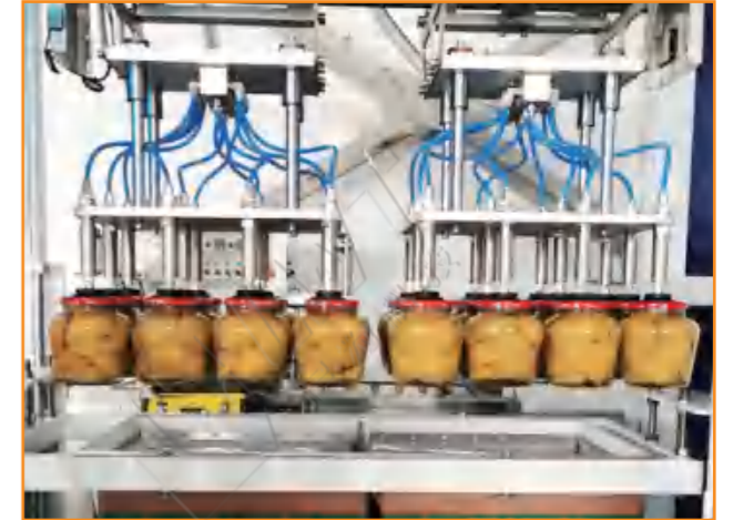
伺服式装箱机(真空吸盘玻璃瓶) Servo packing machine(Vacuum cup glass bottle)
